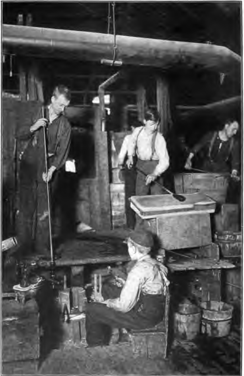
Chautauqua Photographic Co., Pittsburgh BOY HOLDING MOLDS FOR BLOWER IN A SOUTH SIDE GLASS-HOUSE
